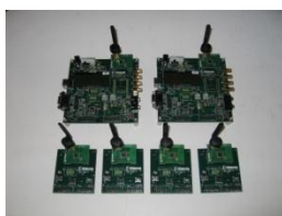
Chipcon CC2431 development kit used to prototype RF-based TOF locationing system.
