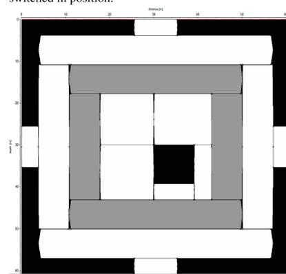
Figure 5: Cross-section model used to evaluate the use of GPR to investigate internal properties of El Castillo with a void. Three internal structures consisting of limestone and sand. GPR transmitter and receiver positioned at opposite sides of the pyramid and incremented at one metre spacing. This is performed for both axes of the two-dimensional model and transmitter and receiver are then switched in position.
