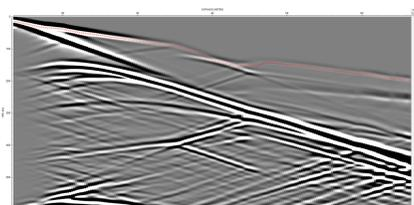
Figure 1: Example of automatic first-arrival 'picking' process of GPR data in ReflexW. First-arrival denoted by red crosses.
