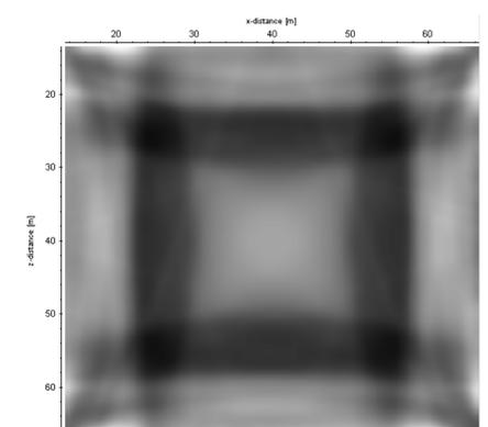
Figure 4: Tomography result obtained from El Castillo scale modelling in ReflexW. Result based on 20 iterations and averaging over 10 points in x and z axes. Three internal structures can be seen by the material boundaries, illustrated by darker and lighter areas.
