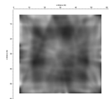
Figure 6: Tomography result obtained from El Castillo scale modelling in ReflexW. Result based on 20 iterations and averaging over 10 points in x and z axes. Three internal structures can be seen by the material boundaries, illustrated by darker and lighter areas.
