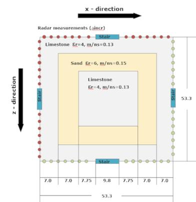
Figure 3: Cross-section model used to evaluate the use of GPR to investigate internal properties of El Castillo. Three internal structures consisting of limestone and sand. GPR transmitter (green) and receiver (red) positioned at opposite sides of the pyramid and incremented at one metre spacing. This is performed for both axis of the two-dimensional model and transmitter and receiver are then switched in position.
